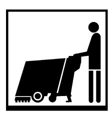
The scrubber-dryer is an automatic machine, push or self-propelled, which washes and dries floors. In the same way as sweepers, scrubber driers can be driven by the operator who follows them on foot (walk-behind machines), they can be equipped with a driver's platform (walk-behind machines) or they can be fully robotized. Within these categories, there are further classifications depending on the washing system, the power supply and the type of traction.
