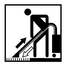
The injection-extraction carpet cleaner is a machine designed essentially to clean carpets and fabrics by dispensing a solution of water and detergent on the surface to be cleaned and the immediate suction of the mixture of solution and dirt. Through a series of nozzles, water or detergent solution (cold or hot) is sprayed on the surface to be cleaned and immediately sucked with the dirt removed.
