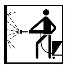
The pressure washer is a machine designed to clean various types of waterproof surfaces, using a high-pressure water jet (cold or hot). To strengthen the cleaning action, the water jet can be combined with detergent or other liquid substances or sanitizing foams as well as abrasive solids.
