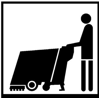
The scrubber-dryer is an automatic machine, push or self-propelled, which washes and dries floors. In the same way as sweepers, scrubber driers can be driven by the operator who follows them on foot (walk-behind machines), they can be equipped with a driver's platform (walk-behind machines) or they can be fully robotized. Within these categories, there are further classifications depending on the washing system, the power supply and the type of traction.
